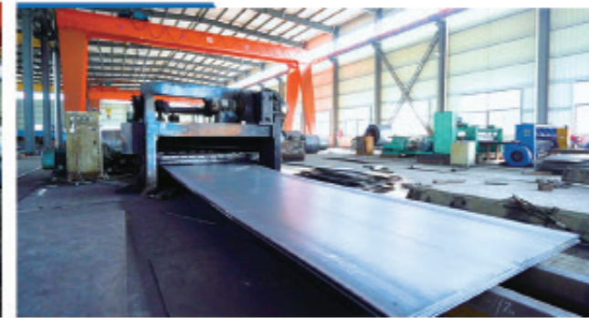
P5 Steel panel cutting
